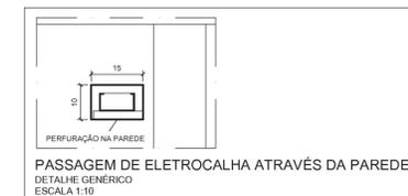
PASSAGEM DE ELETROCALHA ATRAVÉS DA PAREDE DETALHE GÊNÉRICO ESCALA 1:10
